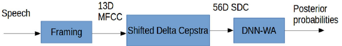
Figure 5: Block diagram of ER system using shifted delta cepstral features
