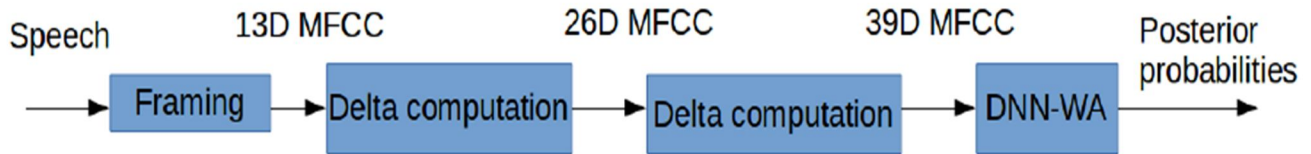
Figure 4: Block diagram of ER system using MFCC dynamic features
