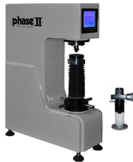
Figure 3: Brinell's hardness tester and micrometer
