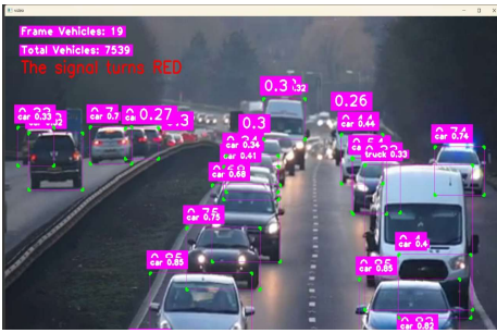
Figure 5: Results Depicting Signal turning RED when the vehicle count is below threshold
