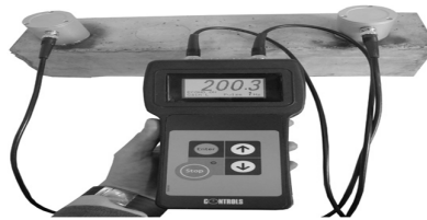
Fig. 6. Ultrasonic pulse velocity test apparatus [13]
