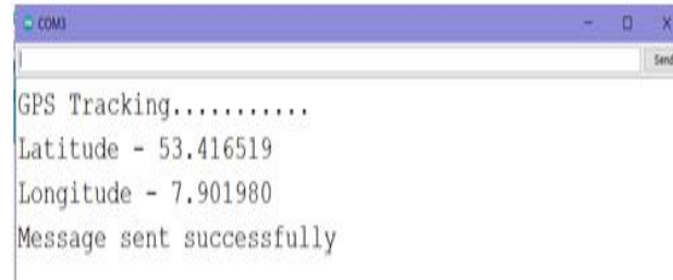
Figure 9. Serial monitor output for tracking location using GPS module
