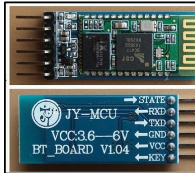
Fig.7 HC-05 Bluetooth Module
