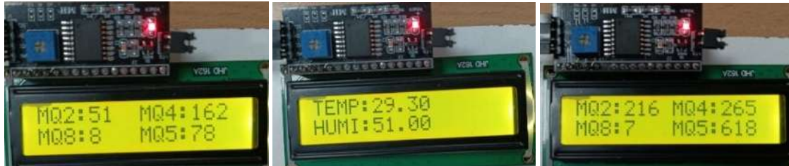
Figure 8. (a) LCD Display Showing Baseline Sensor Values (All Gas Sensors OFF), (b) LCD Display Showing Room Temperature and Humidity values (c) LCD Display Showing Elevated Readings When MQ2 and MQ135 Are ON
