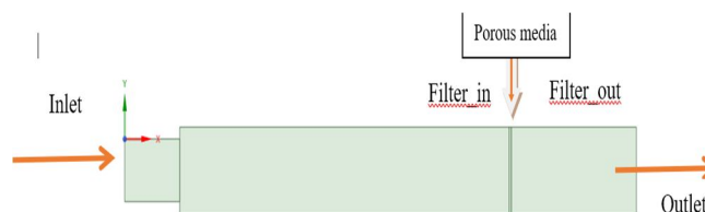
Fig. 2. Geometry of filter test rig
