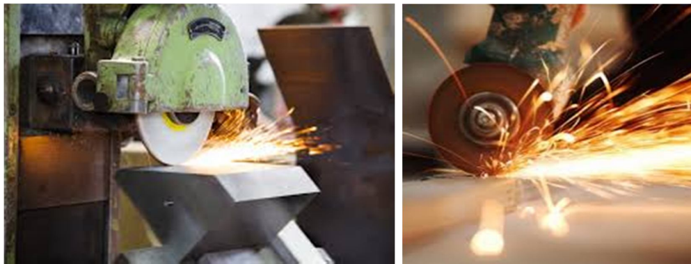
Fig 4. Grinding on welding joint
