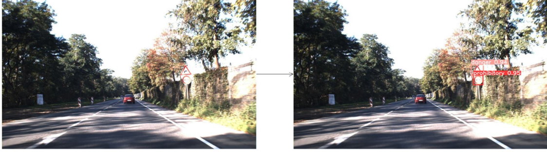
Figure 2: Original Image and Traffic Sign Detected Image using Yolo v5
