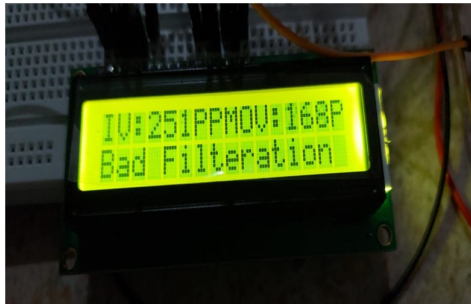
Figure 2. Output display for bad Filtration
