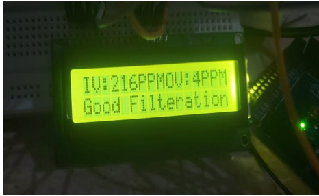
Figure 4. Output display for good filtration
