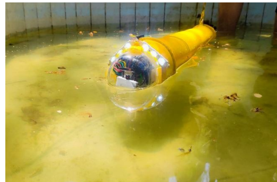
Figure.12. Testing the UUV in stagnant water
