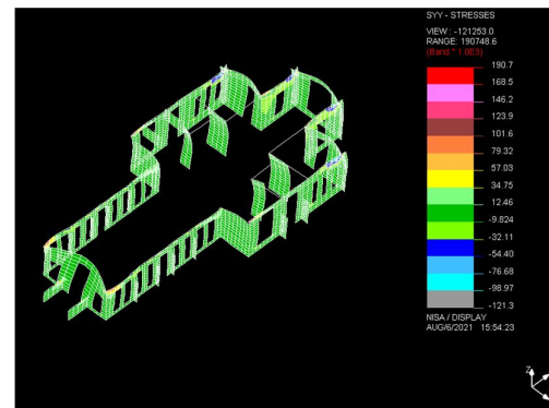
Figure 9. Stress Contour ( S_{yy} ) due to acceleration in y-direction
