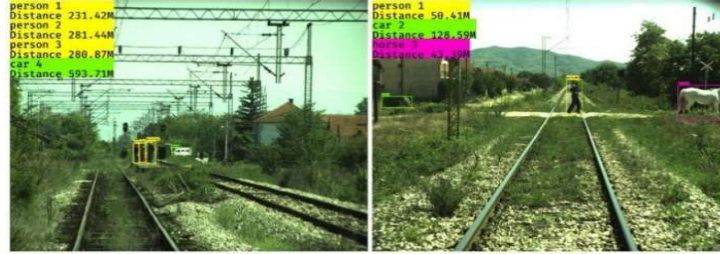
Figure 5. DisNet approximate of distances to obstacle in a railroad site from the RGB camera image
