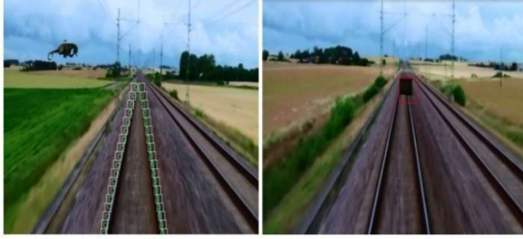
Figure 4. windows-based structured search for obstacle through the discovered railway tracks and digitally added static item and its spotting.
