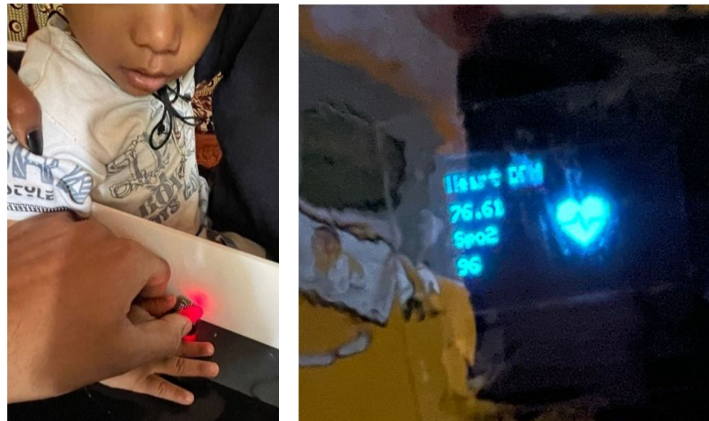
Figure. 12: Baby during the Test process and the results in the OLED
