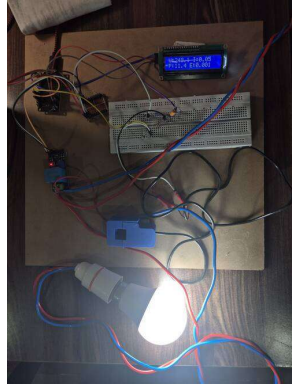
Figure 4. System under test with 9W LED bulb, LCD showing V: 248.1, I: 0.05, P: 11.4
