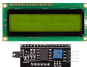
Figure 5. 16x2 LCD Display
