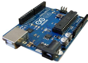
Figure 3. Arduino UNO board
