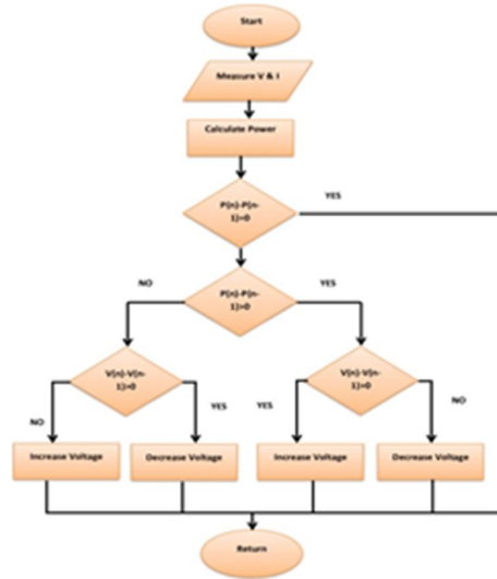
Fig. 3 Flowchart of Perturb & Observe algorithm
