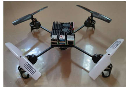
Fig 5: Fully assembled Aero Flame Drone prototype during stability testing.
