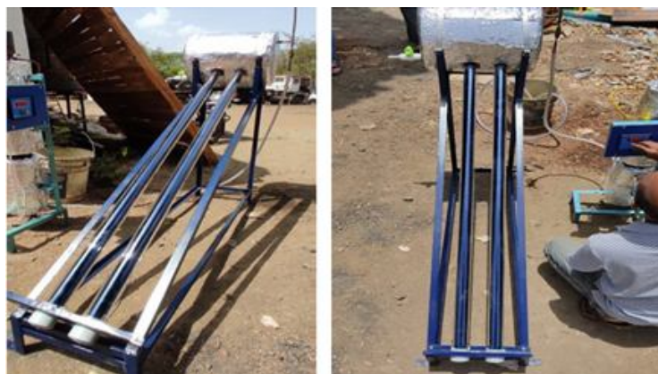
Figure: 4. Solar water heating section
