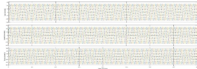
Fig 11. Waveforms for Load current, injected current, Source current
