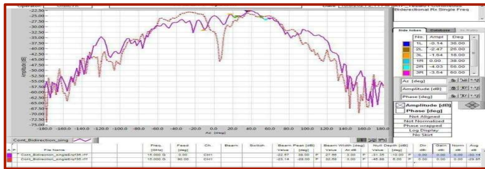
Figure 6. Radiation pattern (Cartesian coordinate system) at 15 GHz
