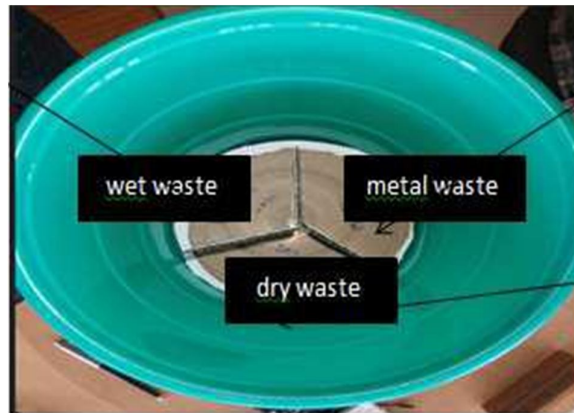
Figure.7. Hardware setup of Smart bin
