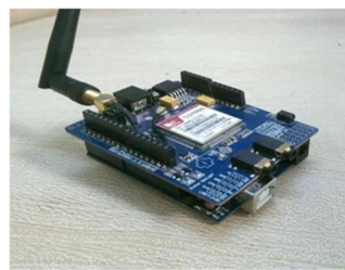
Figure 6. GSM module with Arduino
