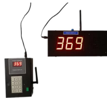
Fig. 2 : An example of a wireless display system
