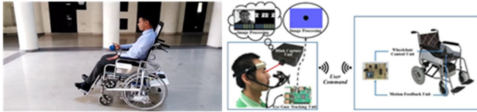
Fig. 2 : Prototype of the wheel chair (Similar one will be designed & built by us) & Eye blink sensor design (Similar one will be designed & built by us)
