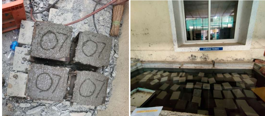
Figure 2: Casting of concrete cubes to be embarked on mechanical testing using recycled Sand.
