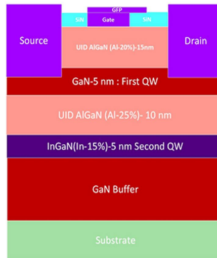
Figure 1: Double quantum well EMODE structure with GFP and SiN passivation layer
