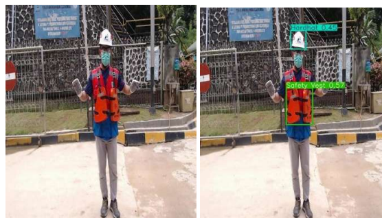
Fig. 6. Detection output of multiple safety equipment
