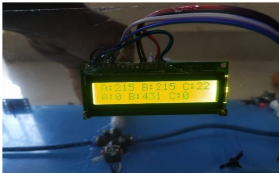
Figure 6. LCD display showing the gas and pressure sensors readings
