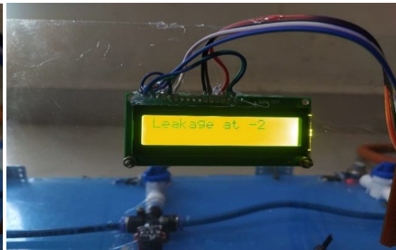
Figure 7. LCD display showing the position of leakage
