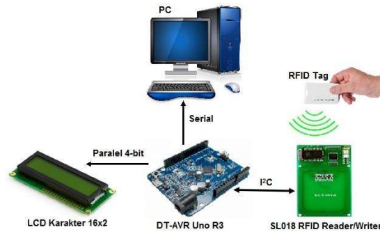
Fig.2: System Architecture of RFID Equipment Tracking System
