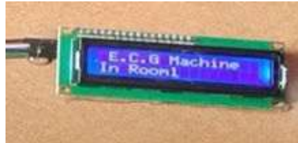
Fig.8: GUI output indication of the detected room status
