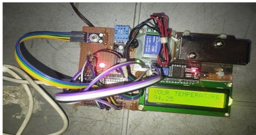
Figure 2: Temperature shown 94.25°F below the range which have been fixed up to 100°F
