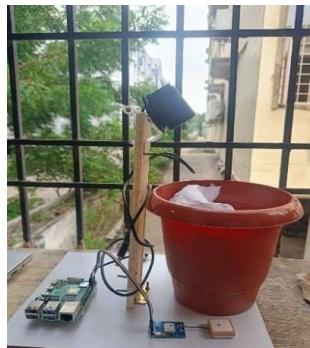
Fig.6. Completed AI-powered smart garbage bin Assembly
