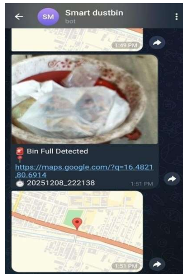
Fig.7. Bin Full Alert with GPS Notification
