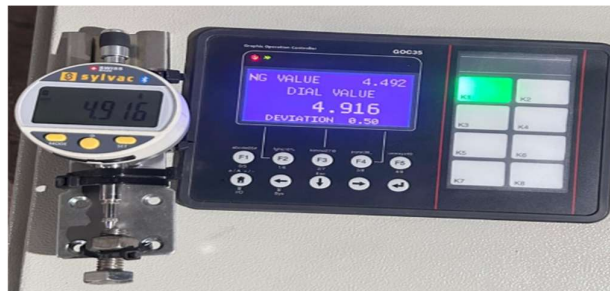
Figure 4: Basic PLC panel and dial Set up (Actual Photograph)
