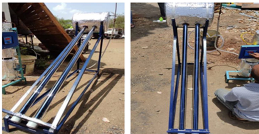
Figure 4: Solar water heating section
