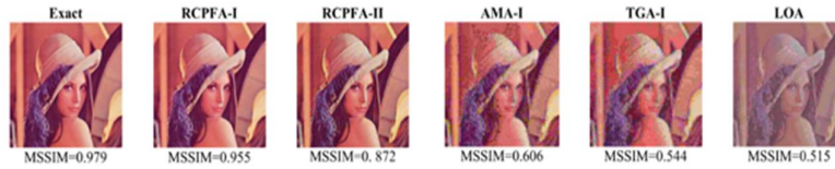
Figure 3. Output images for DCT circuits using different FAs [10]
