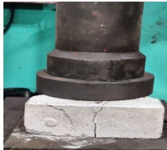
Fig.2 Compressive strength test of paver block
