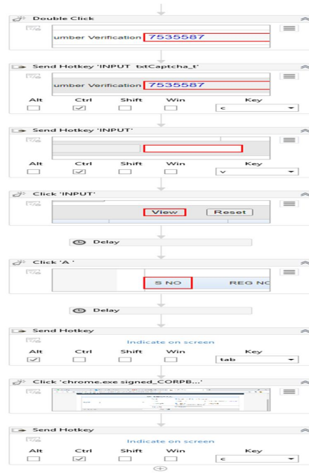
Fig 5 Sequence of automation on generating certificates
