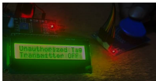
Figure 5. Transmitter status when unauthorized card is tapped
