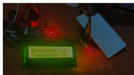
Figure 4. Transmitter status when authorized card is tapped
