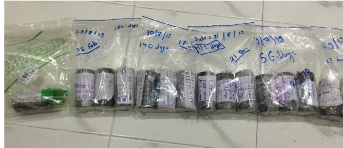
Fig. 3. Cured UCS sample of an untreated and optimum mix
