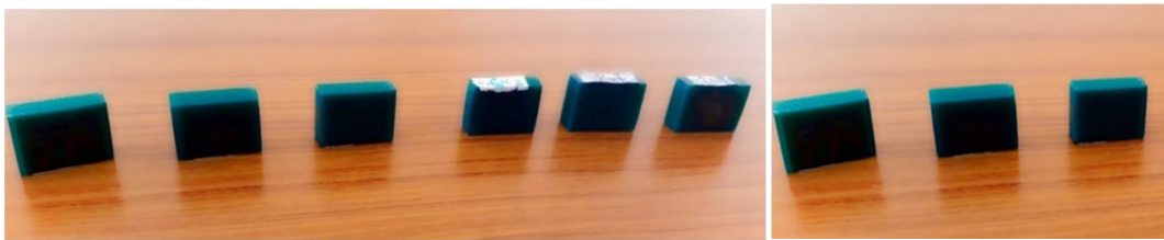
Fig. 1: Specimens built on FDM Machine
