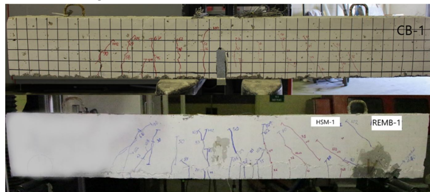
Figure 9-Crack Propagation in CB and REMB
