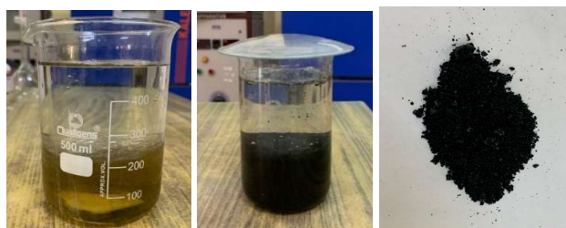
Figure2: Base solution prepared using precipitate method.
