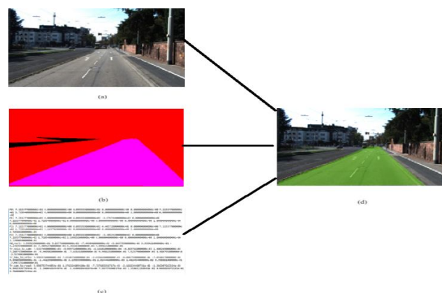
Figure 5. Drivable road segmentation a) Raw image b) Segmented Mask c) Annotation d) Corresponding result
