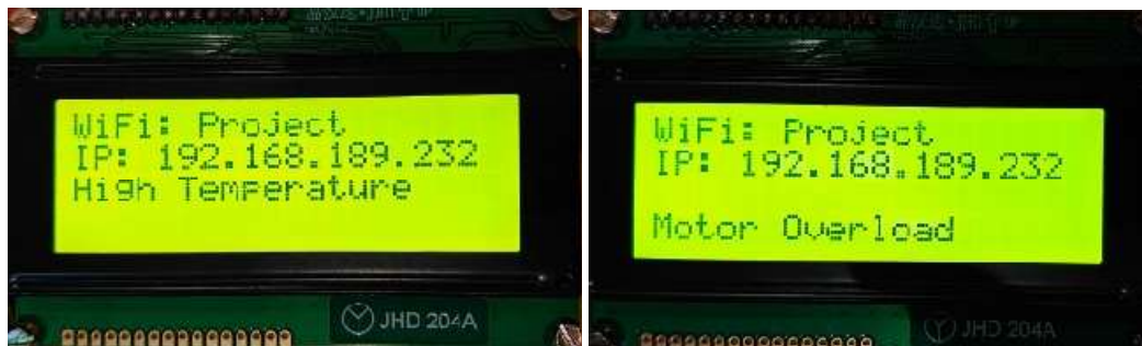
Fig.4 (a). High Temperature Fault in motor
