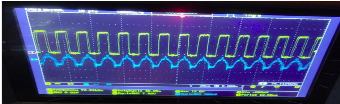
Fig. 16. the gate signal and current waveform at input inductor
