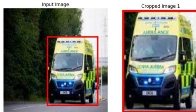
Fig. 6. Emergency Vehicle Cropped after Object Detection, Fed into CNN for Further Classification
