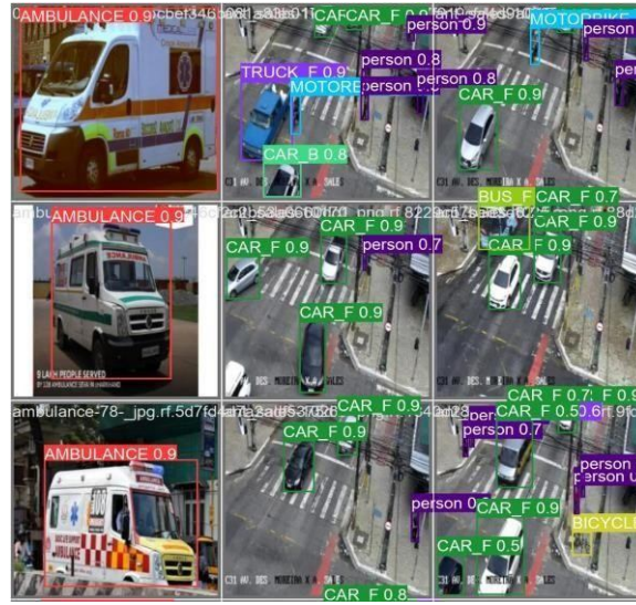
Fig. 6. Different Classes of Vehicles Detected by Yolov8
