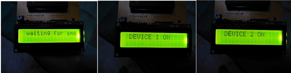
Figure 5. Status displayed on the LCD for the above commands taken as instances
