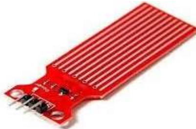
Figure:3 Water level sensor
