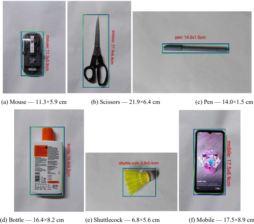
Fig. 4. Detection outputs of each person in individual: cyan boxes = A4 reference sheet; green boxes = detected objects with W×H (cm) written in red. All samples within 0.20cm of vernier caliper reference.
